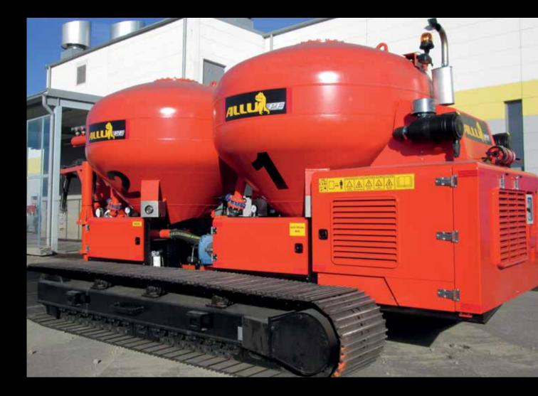
The mobile ALLU Pressure Feeders are high capacity, tracked, intelligent feeding units for dry binders. The computer-controlled binder feed prevents any unnecessary amount of binder to be feed. This unique feature brings big cost savings and efficiency to any jobsite.
