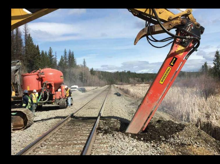
The ALLU Processor is a power mixer hydraulic attachment for excavators. This attachment converts the excavator into a powerful and versatile mixing tool, capable of penetrating and mixing a variety of difficult materials - everything from clay, silt, peat and dredged sediments to hazardous liquid waste and contaminated soil.
