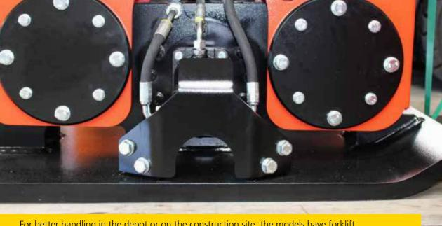
For better handling in the depot or on the construction site, the models have forklift mounts to ensure easy and safe transport.
